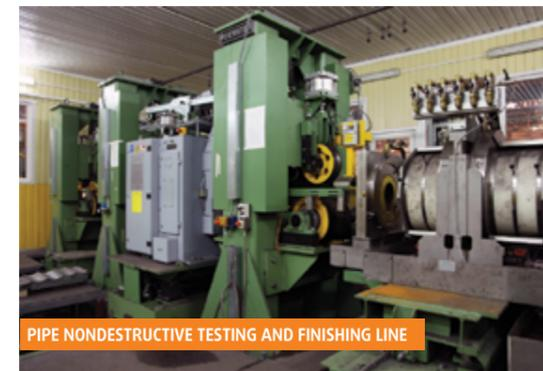
PIPE NONDESTRUCTIVE TESTING AND FINISHING LINE
