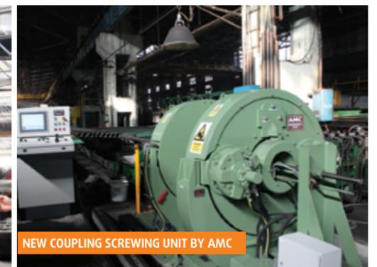
NEW COUPLING SCREWING UNIT BY AMC
